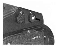
The AE lock button is useful when intentional over- or underexposure is desired for special effects, etc., or under difficult lighting conditions. The shutter speed indicated by the exposure meter needle in the viewfinder is held when the AE lock button is pressed. As long as the AE lock button is pressed, the shutter speed will remain the same even when the camera is pointed at a brighter or darker subject.
