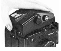
1. To attach the AE Prism Finder to the camera body, lift up the front part of the finder slightly and place the rear part on the camera. Next, press down firmly but gently on the front part of the finder and the locks will automatically engage to hold the finder securely in place.
