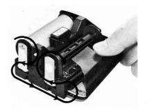
**5.** Gently pull out some of the leader paper, pulling it over and around the pressure plate. Then insert the tip of the leader paper into the slot of the take-up spool.
