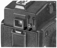
Simultaneously press the safety button (C) with the right hand and the finder release button (D) with the left hand. Next, remove the finder by lifting upward.
