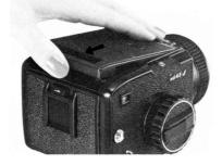
Remove the upper body cover from the camera by sliding it to the rear and lifting up.
