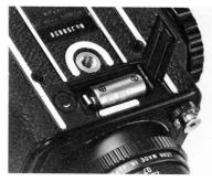
2. Next, align the ⊕ ⊖ marks of the battery with those indicated in the battery chamber. Then insert the battery and close the cover.
