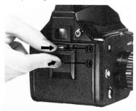
While gently pushing in on the memo clip (16), move the back cover latch (14) in the direction of the arrow and the camera back cover will open.
