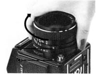
While aligning the two alignment dots (31 & 4), insert lens into camera body. Then twist lens clockwise until it clicks and locks into place.
