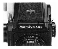
When the battery check button (19, located above the film advance knob) is depressed, the battery check lamp (7, located above the shutter speed dial) illuminates. If the battery check lamp fails to go on, it is time to replace the battery.
