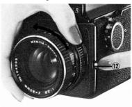
While depressing the lens release button (12), grasp the part of the lens barrel that has the depth-of-field scale (30) and alignment dot (31), and twist the lens counterclockwise until it stops. Then lift out.
