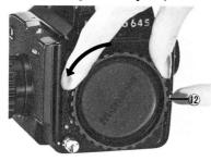
While depressing the lens release button (12), turn body cap counterclockwise until the red dots are aligned and lift out.
