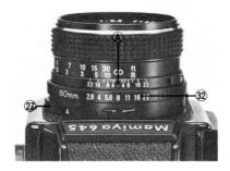
Set the desired f/stop on the aperture ring (32) by aligning the f/number with the red reference dot (A). (The aperture ring has a click stop for each f/stop. In-between clicks can also be used.)
