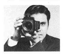
When hand-holding the camera with the waist-level finder attached, adjust the length of the neck strap to take up all slack and support the camera gainst the body. As accessories, Mamiya offers a selection of hand grips which not only help to eliminate camerashake, but are also convenient for carrying the camera.
