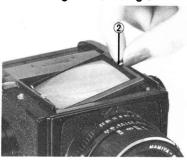
Insert the two tabs of the focusing screen into the slots at the back of the opening in the camera top and press lightly so that the screen clicks into place.
